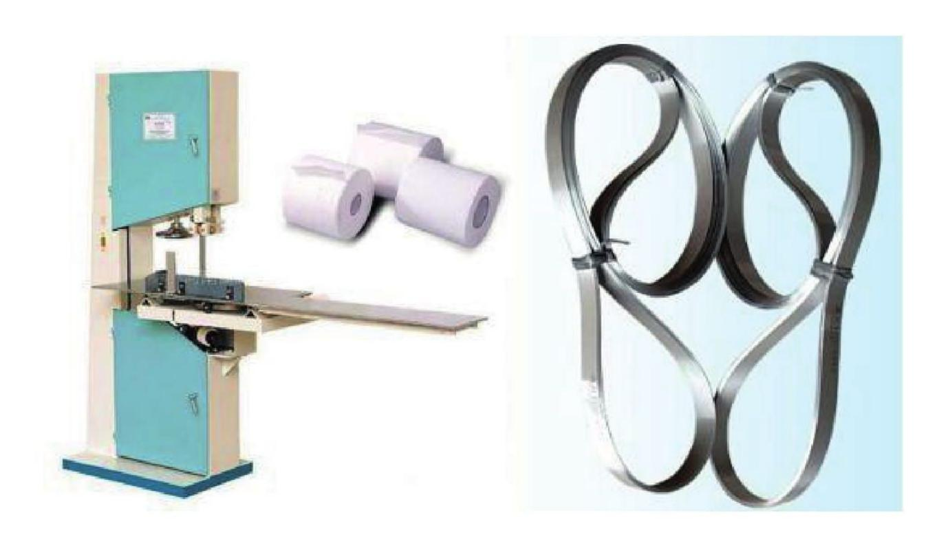
Manual band saw machine for toilet paper roll cutting
